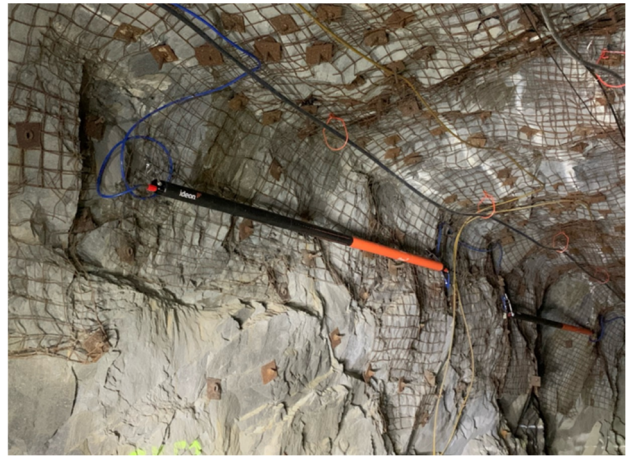
Figure 6 Ideon borehole muon detector installed in-mine.
